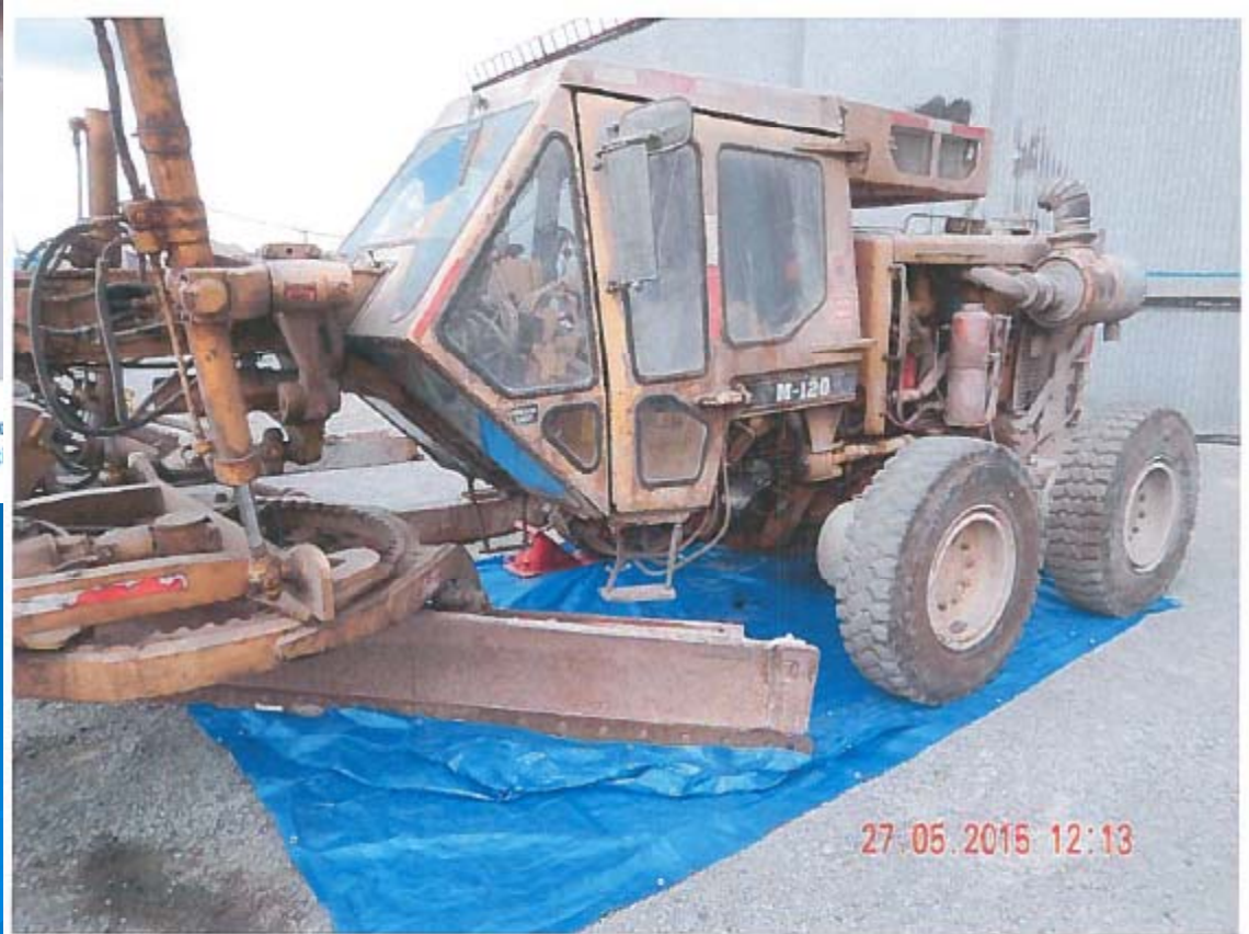
Photo 6 – Mechanical Shop 2 Building 51 – Equipment being parked outside the shop are placed on tarps as temporary containment to catch leaks.
